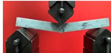
Figure 1. The crack propagation in sample 16a
